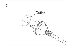
**DANGER:** Improper connection of the equipment-earthing conductor can result in an increased risk of electric shock. Check with a qualified electrician or serviceman if you are in doubt as to whether the product is properly earthed. Do not modify the plug provided with the product—if it will not fit the outlet, have a proper outlet installed by a qualified electrician.
